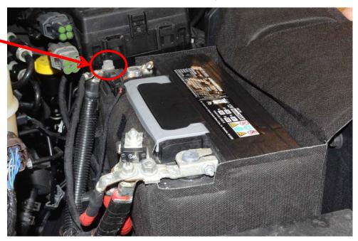
If a high amperage cable (with a thick ring terminal) is to be installed on the left side battery B- connector, the OEM nut shown above can be replaced with a thinner nut. Use part number 06502720 (available from Mopar) which is 3mm thinner. Torque to 11.0Ft/Lbs. (± 2.0Ft./Lbs.).
