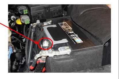
Right (Passenger) Side Battery B+ Connector Do not install wiring / terminals of any kind at these locations
